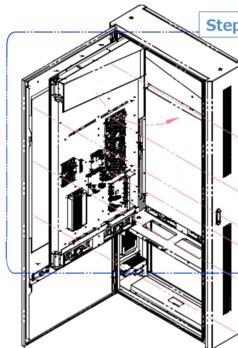
Step-4, Remove the LCD Panel
